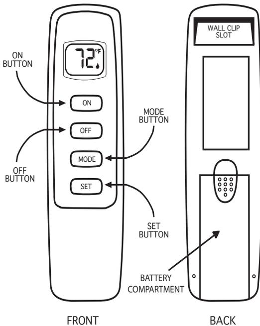
This remote control SYSTEM offers the user a battery-operated remote control that operates most millivolt gas valves used in some heater rated gas logs, gas fireplaces and other gas heating appliances.
