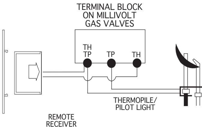
Operation of the remote receiver is similar to that of a thermostat in that both turn the gas valve ON and OFF based on input signals. A thermostat's input signals are different temperatures. The remote receiver's input signals come from the transmitter.
